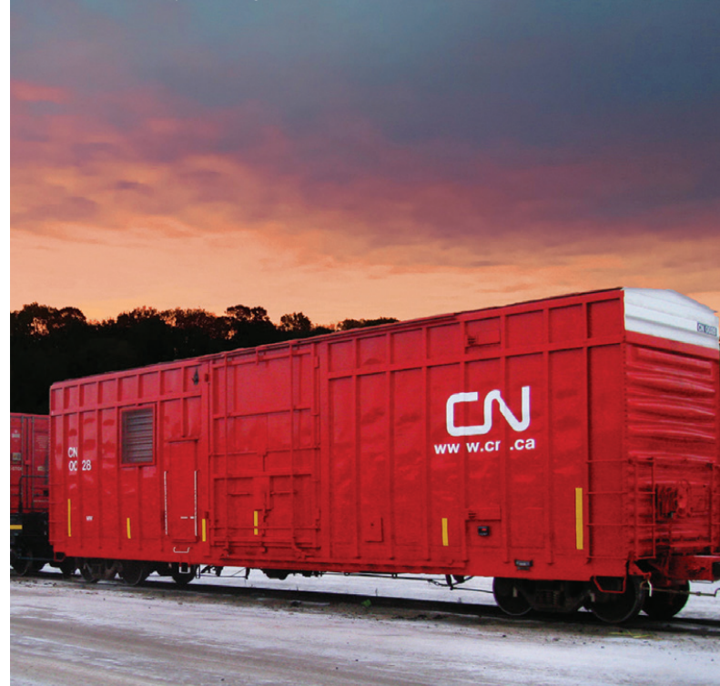
CN's distributed air braking cars supplement the air supply to a train's air brake system during colder weather.
