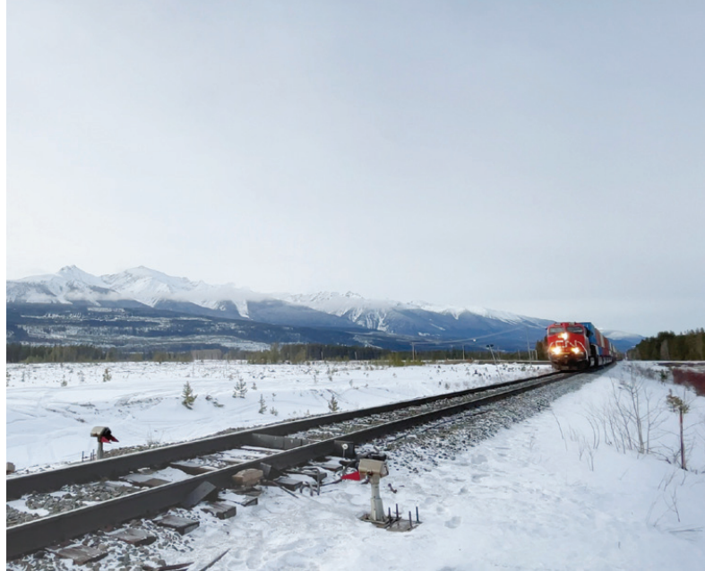
Wayside detectors in foreground stand ready to inspect approaching CN train in Blue River, BC.
