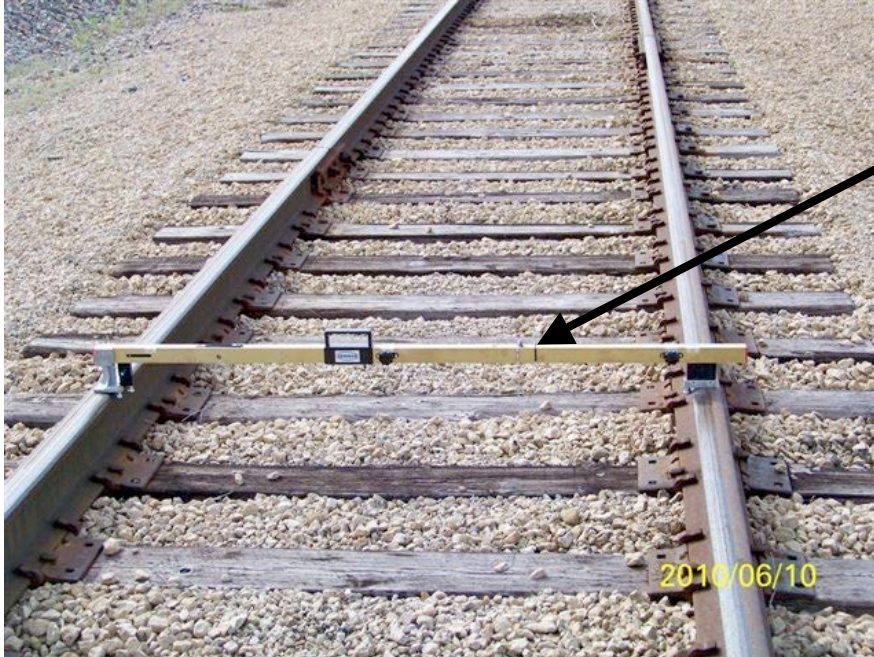
(Figure 3: Measuring gauge with a gauge measurer)
