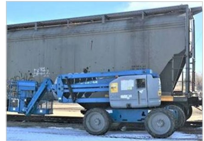
Figure 2. Fall protection - articulated boom ladder
