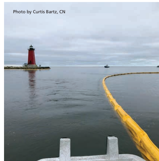
CN conducted a containment boom deployment exercise in the swift currents of the Manistique River to prevent any potential diesel fuel from the "derailed" locomotives from entering Lake Michigan.
